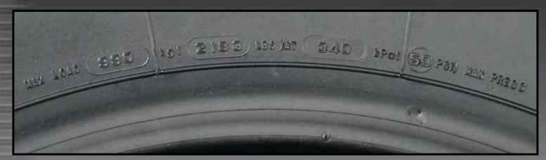
MAX LOAD 990 kg (2183) LBS AT 340 kPa (50 PSI) MAX. PRESS.
