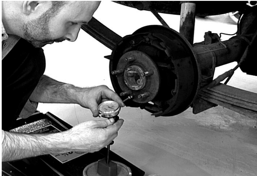
Measuring Hub/Flange Face Runout
