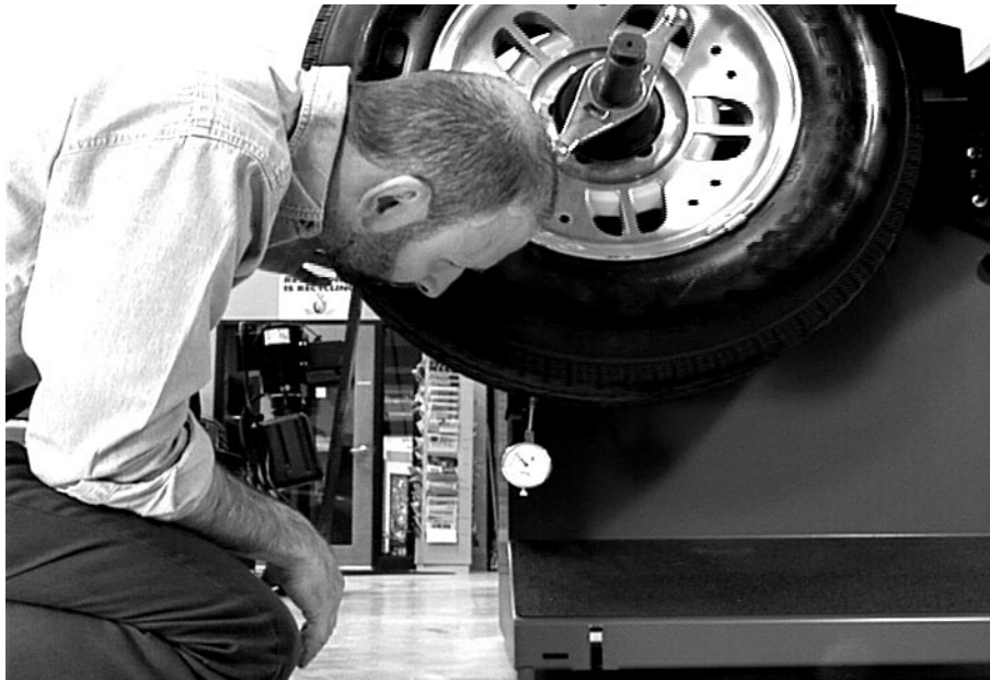
Measuring Radial Runout of the Tire/Wheel Assembly
