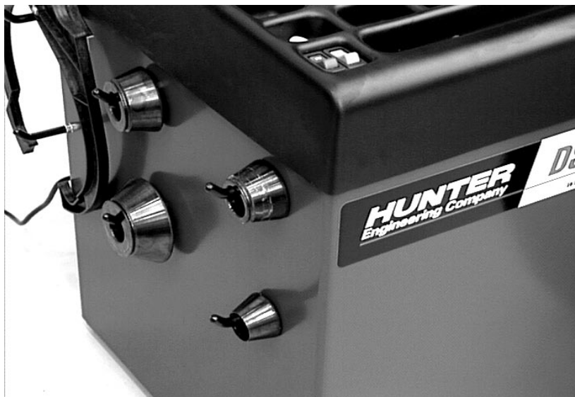
Spin balancers come with assorted centering cones to accommodate the many variations found in the size of wheel center holes.
