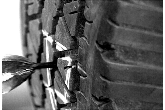
Trimming the rubber stem of a two-piece repair unit.
