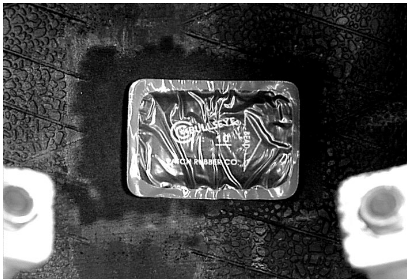
Preparing for final installation of a two-piece repair unit.
