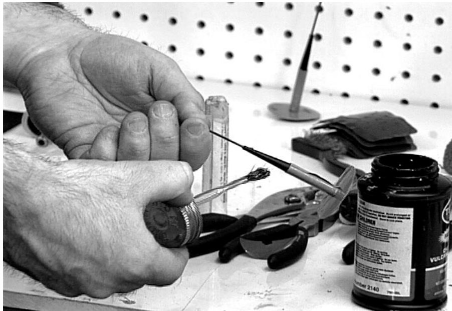
Preparing a one-piece combination repair unit for installation.
