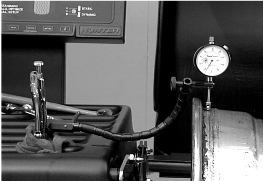
Measuring Radial Runout of the Wheel
