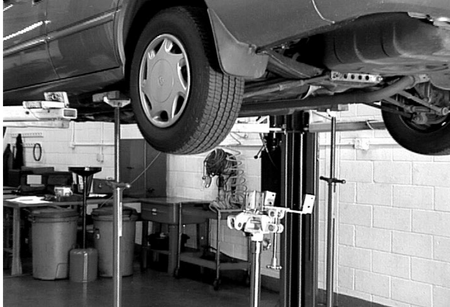
High-reach jack stands are often used to support the vehicle during major underbody repairs, such as removing the fuel tank.
