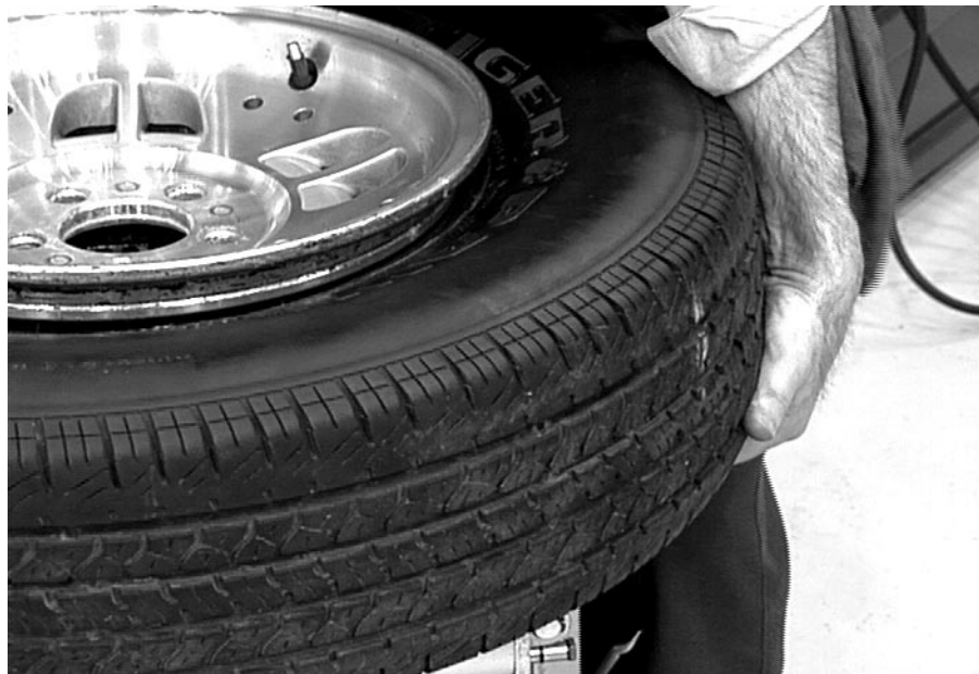
Indexing is a procedure in which the high spot of the tire is aligned with the low spot on the wheel.
