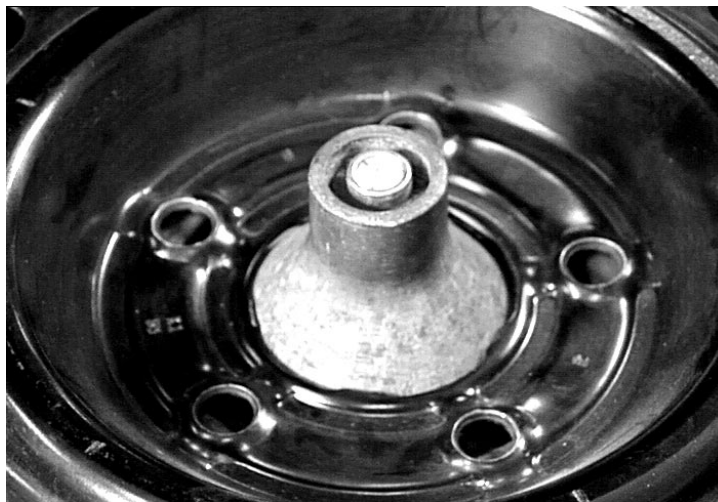
A bubble balancer is designed to statically balance the tire and wheel assembly.
