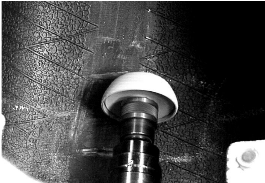
Buffing the innerliner is necessary to remove the mold marks and provide a smooth uniform surface for the repair unit.
