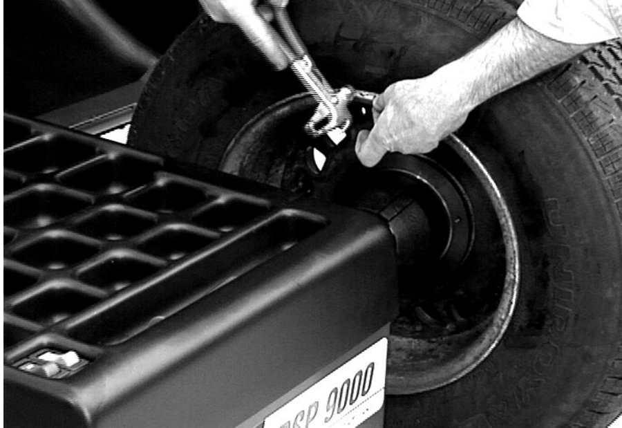
Clip-on weights are installed at the TDC position using a special hammer.
