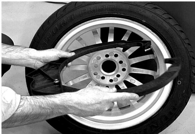
A caliper is used to measure the width of the rim, as well as the internal diameter of the wheel when necessary.
