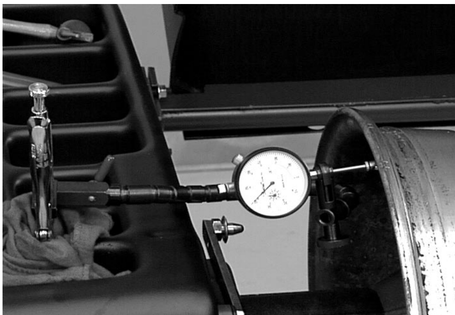
Measuring Lateral Runout of the Wheel
